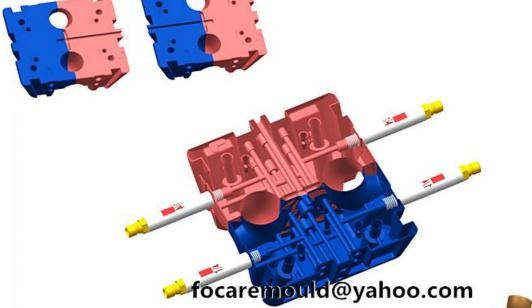
collapsible core slides & cooling
